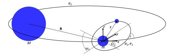
FIG. 1. The hierarchical three-body problem, in which  $|\mathbf{r}| \ll |\mathbf{R}|$  (the figure is not to scale).
